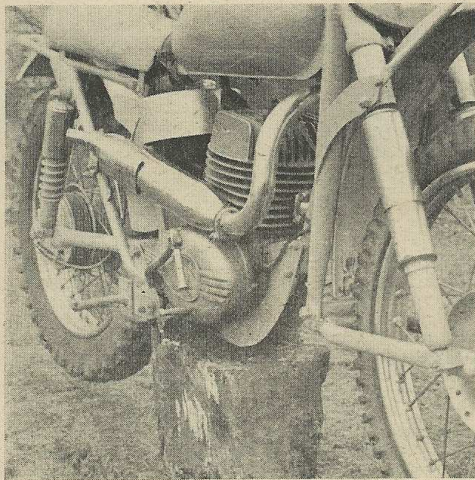
Two close-ups of the engine, which also show the unusual route taken by the exhaust pipe.
