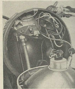
Complex switchgear wiring-harness details. But this equipment was quite trouble-free during 3,500 miles. Note detachable key to ignition switch.
